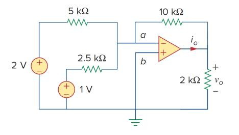
Summing/Difference Amp.  $\bigcirc \bigtriangledown \bigcirc \bigcirc \bigcirc \bigcirc \bigcirc \bigcirc \bigcirc$
