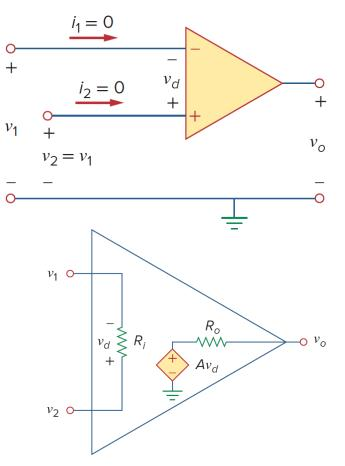
A 741 op amp has an open-loop voltage gain of  $2 \times 10^5$ , input resistance of 2 M $\Omega$ , and output resistance of 50  $\Omega$ . The op amp is used in the following circuit. **Using the ideal op amp model**, calculate the closed-loop gain  $v_o / v_s$ . Find  $i_o$  when  $v_s = 1$  V.
