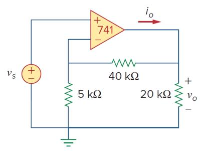
Using the ideal op amp model, determine the output voltage  $v_o$  in the circuit.
