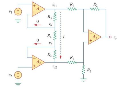
$v_o = \frac{R_2}{R_1} \left( 1 + \frac{2R_3}{R_4} \right) (v_2 - v_1)$
