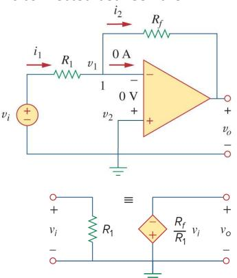
(inverting amplifier's equivalent)
