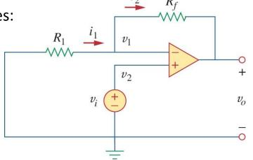
• There is once again negative feedback in the circuit, thus,  $v_1 = v_2 = v_i$ . This gives:
