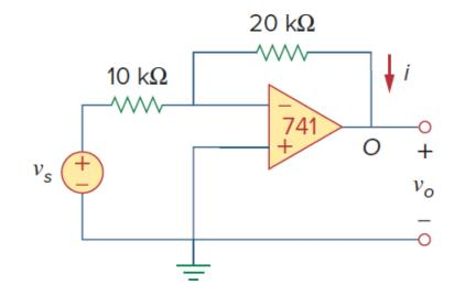
If  $v_i = 0.5$  V, calculate: (a) the output voltage  $v_o$ , and (b) the current in the 10-k $\Omega$  resistor.
