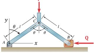
(2) Draw the system when it undergoes a **positive** virtual displacement  $\delta q$  [here:  $\delta q \equiv \delta \theta$ ].
