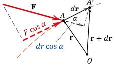
This can be considered as either the component of the force in the direction of the displacement times the displacement, or the component of the displacement in the direction of the force times the force.
