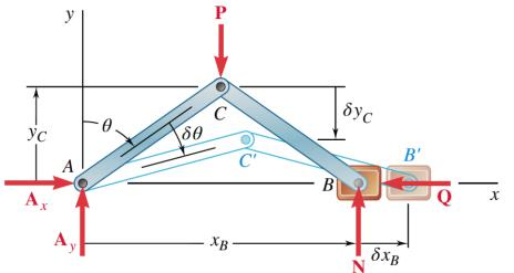
Note: The total work of the internal forces at the connections (like *C*) is <u>zero</u>; Moreover,  $\delta U_{\text{Reactions}} = \delta U_{A_x} = \delta U_{A_y} = \delta U_{N} = 0$ . Thus, only **P** and **Q** do work in this virtual displacement.
