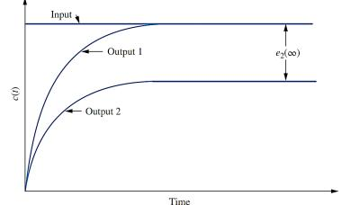
• If N = 0, then  $K_p = z_1 z_2 \dots / p_1 p_2 \dots$  and there is a <u>constant steady-state error</u> (Output 2).
