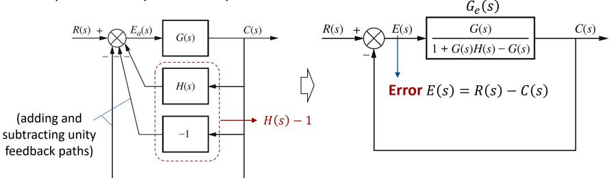
After converting a nonunity feedback system to an equivalent unity feedback system, we can use previous methods for  $G_e(s)$  for finding the Steady-State Error  $e(\infty)$ .
