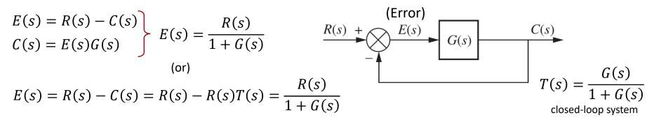
Note: You should always first make sure the closed-loop system T(s) is stable, using a method like the Routh-Hurwitz criterion.
