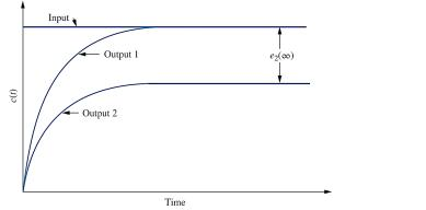
**Note**: Errors are measured **vertically** between the input and output as  $t \rightarrow \infty$ .
