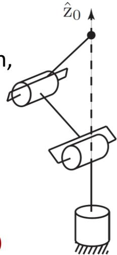
Assume that the joint axes  $(S_4, S_5, S_6)$  of the spherical wrist are aligned in the  $(\hat{z}_s, \hat{y}_s, \hat{x}_s)$  directions, respectively:
