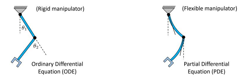
In obtaining a mathematical model, we must make a **compromise** between the **simplicity** of the model and the **accuracy** of the results of the analysis. We may simplify the system model in order to design a relatively simple controller.
